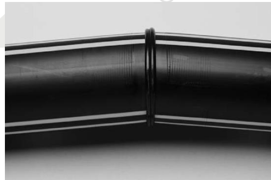
Improper alignment in fusion machine—mitered joint.
