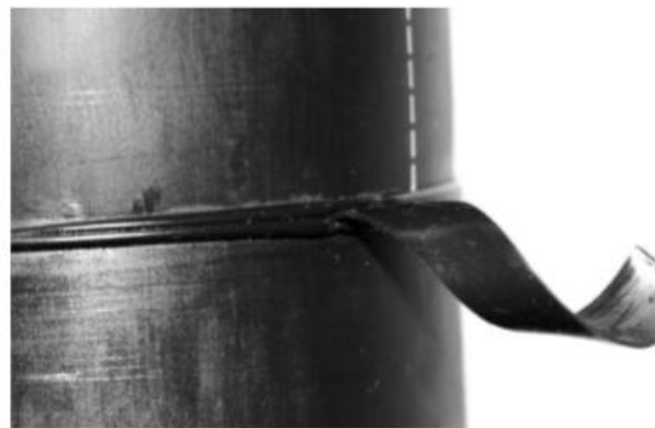
Improper alignment in fusion machine—mitered joint.
