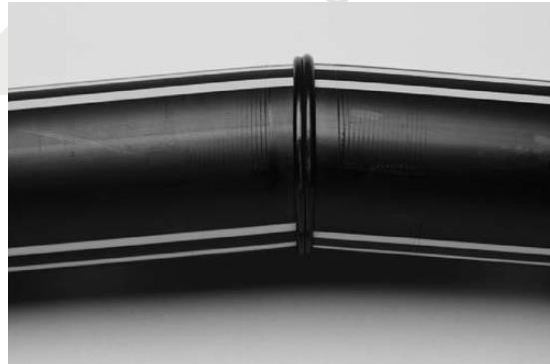
Improper alignment in fusion machine—mitered joint.
