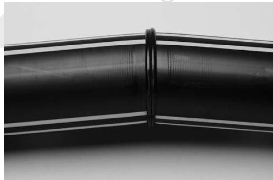
Improper alignment in fusion machine—mitered joint.
