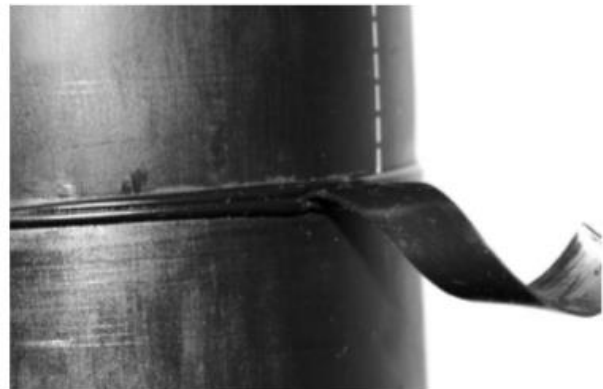
Improper alignment in fusion machine—mitered joint.
