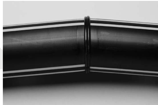
Improper alignment in fusion machine—mitered joint.
