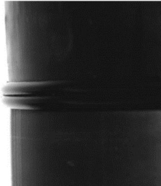
Proper double roll-back bead. Proper alignment.
